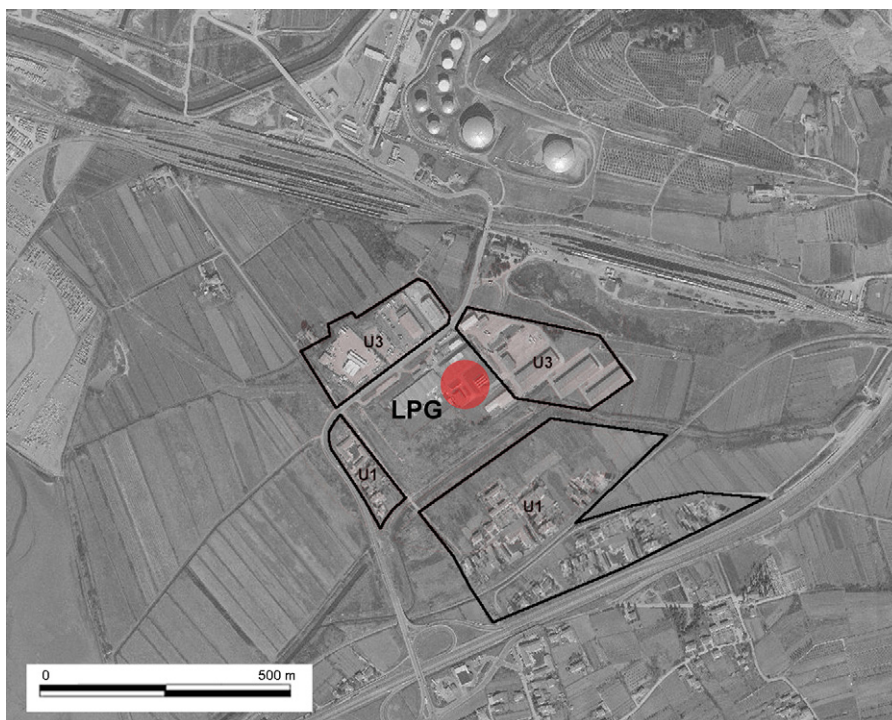
Fig. 13. Illustration of possible land development scenario after elimination of the BLEVE scenario. Explanation of U1 and U3 is in Table 5.
